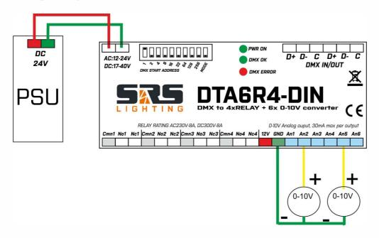
By default, the first 4 DMX channels are RELAY 1-4 and then another 4 DMX channels are analog outputs 0/+10V. Switching relay from 0 to 100% is performed by the value of 25 on the DMX channel according to the DMX start address setting. Without power, the CMNx and NCx contacts are closed
