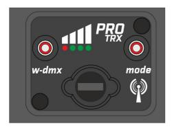
2. W-DMX is ready to be linked, DSR8W works as splitter until the W-DMX signal is coming to the W-DMX port. Signal bargraph is showing the signal strength.
