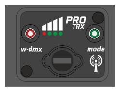
3. W-DMX linked + DMX is missing on Transmitter. The W-DMX LED is changing from red to green slowly and Bargraph is working.
