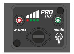
4. The W-DMX is linked to the Transmitter and receiving the DMX signal. Both indicators are green. Bargraph is working.
