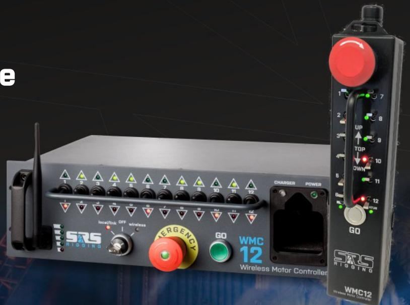
**WMC-G3** is a new generation of Wireless Hoist Controllers with WMC HAND with external antenna. This new external antenna solves all the issues of previous versions and therefore provides its user with easy and trouble-free operation with even wider range of wireless signal.
